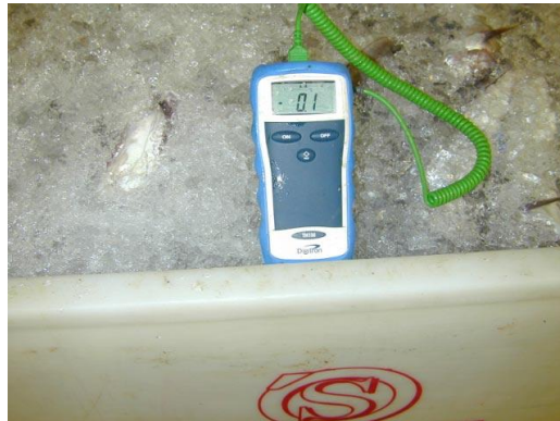
Figure 3: Measurements from Fishgates employees showed a temperature in the flesh was around 0°C
